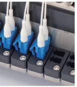
Polishes up to 24 connector plugs. And the individual pressure system lets you polish as few as 1 at a time. Besides connector plugs, it can do specialized polishing such as all types of ferrule and bare fiber.
