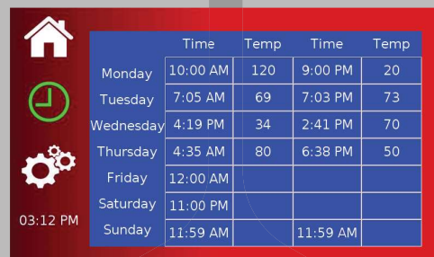
Schedule feature allows program of oven temperature to start at predefined times and also as a safety feature if unit is left on after a shift has been completed
