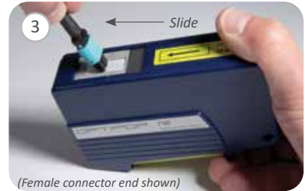
3 (Female connector end shown) Keep connector perpendicular to cleaning surface
