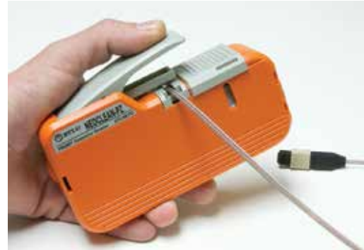
Cleaning PRIZM® LightTurn® connector
