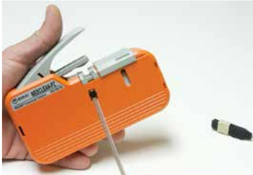
Placing PRIZM® LightTurn® connector into cleaner
